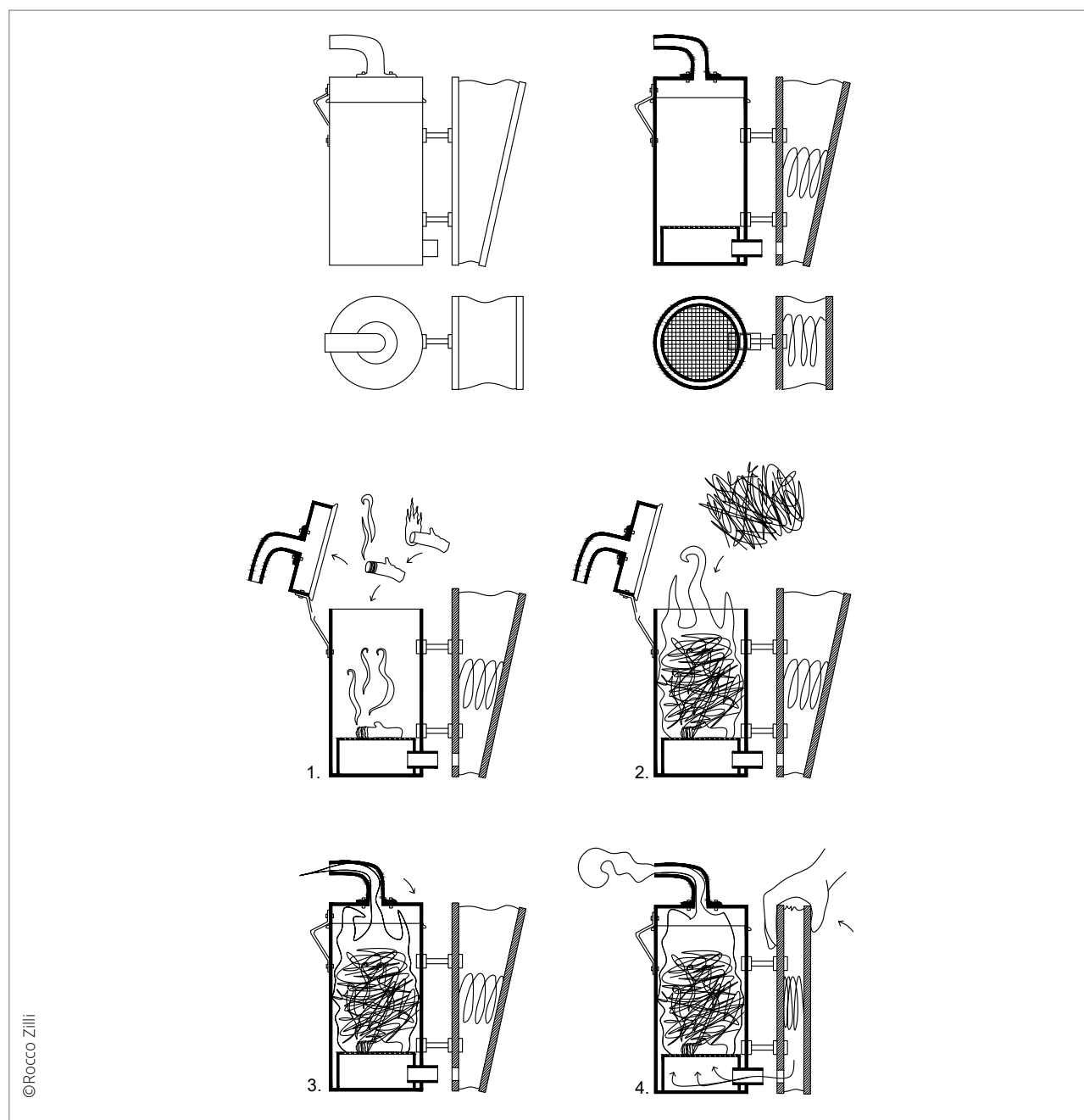
Figure 4: Lighting the smoker and creating smoke
