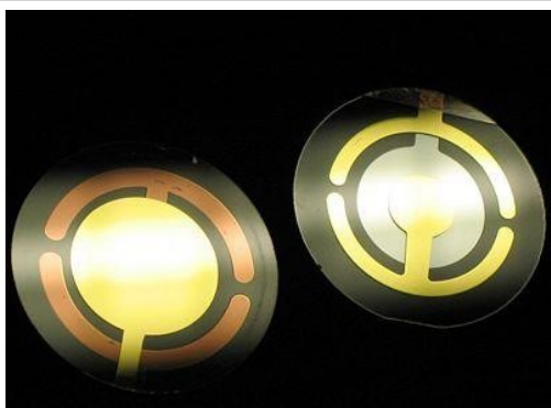
Photograph of typical quartz crystal resonators as used for QCM, metalised with gold electrodes (left: front electrode, right: back electrode) by vapor deposition (from Wikipedia).
