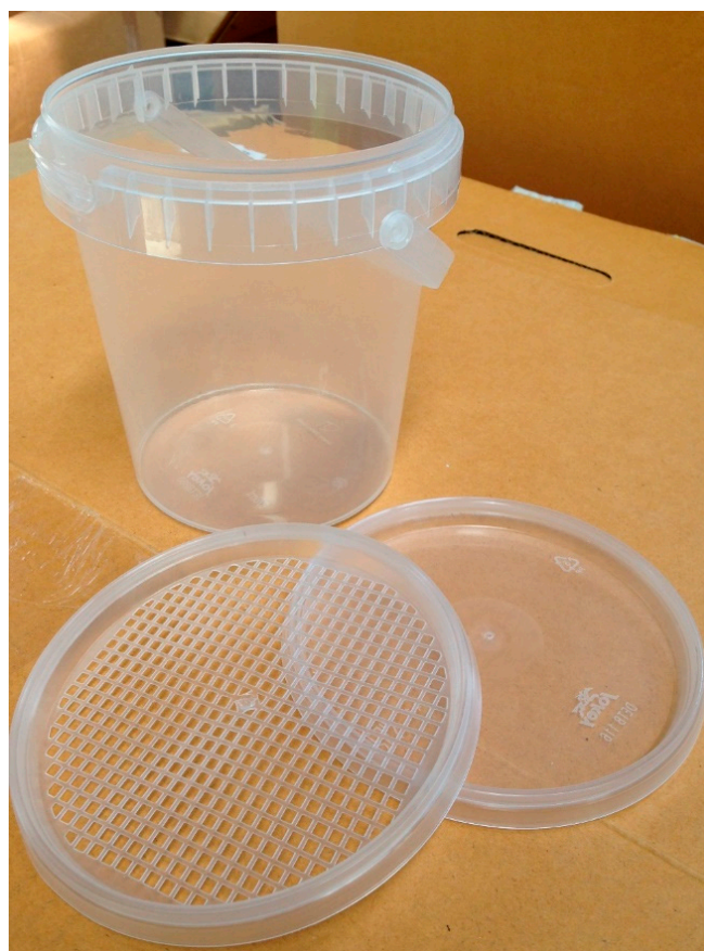
Figure 1. Jar provided with a mesh to separate powdered sugar and mites from adult bees.
