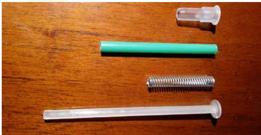
Photo 4. Components of the beebread collector: spring, plunger, little rigid tube, plastic conical support.
